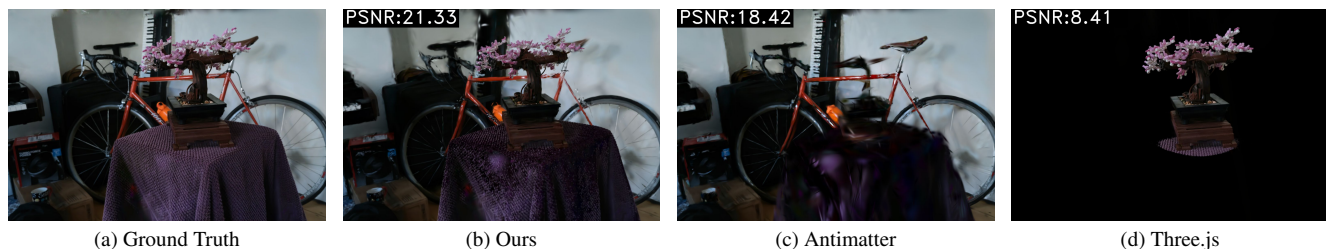
Figure 4. A concrete comparison between the three aforementioned methods on the bonsai scene taken from Mip-NeRF360 indoor scenes being rendered at 10% splats compared to the ground truth. Notice how both the bonsai and cloth are being rendered at a higher quality in Ours(b) than in Antimatter(c). Tree.js(d) will almost always be outperformed using standard metrics as the background is completely missing.
