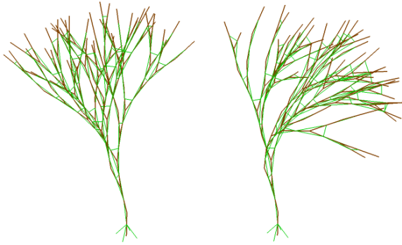
Figure 2: A tree skeleton with a mass-spring system attached to it. Linear springs are drawn in brown, angular springs in green. Left: system in its rest state. Right: wind causes the skeleton to bend towards the right side.
