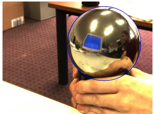
Figure 6. Locating the spherical mirror: robust ellipse detection.
