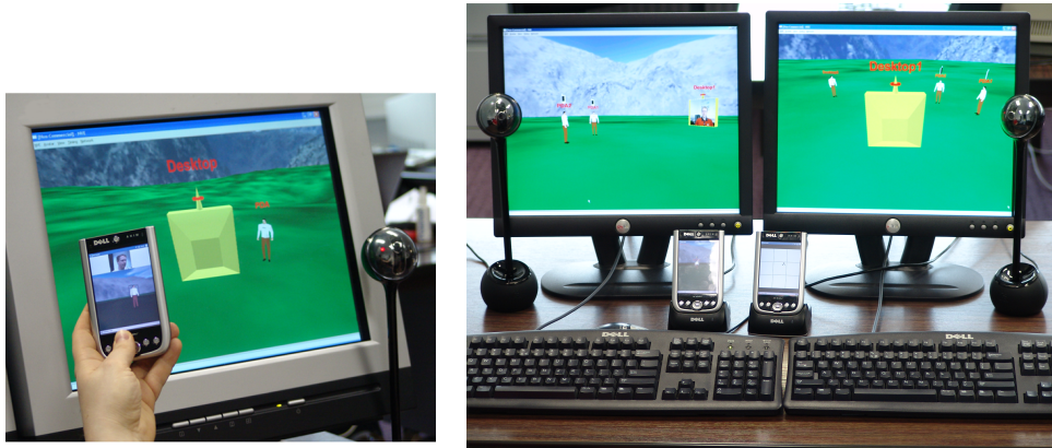
Figure A.10: Example ALVIC multi-platform setups including standard desktop clients as well as mobile Dell Axim x51v PDA devices.
