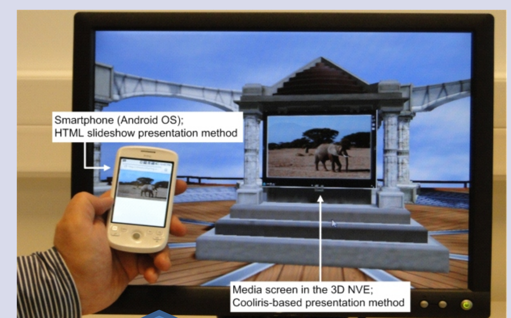
Example cross-platform sMS session (picture sharing scenario involving a desktop PC and a smartphone)
